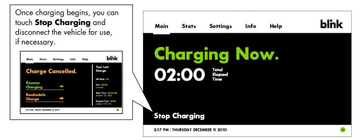
**Note:** The **Total Elapsed Time** indicates the cumulative time that the vehicle has been drawing current from your **blink**. To determine whether your vehicle has a full charge, check its onboard charge status.
